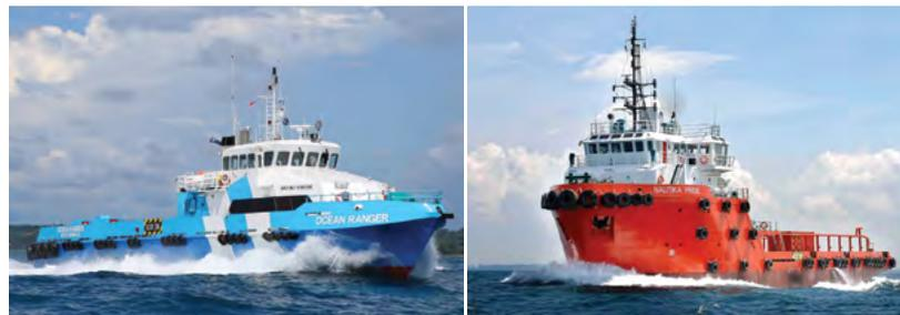
Above left: 38-metre, 4,500 hp triple-screw fast crew boat built by Sarawak Slipways with one Cummins KTA50 and two KTA38 main engines, and two Cummins 6BT5.9 gensets.
