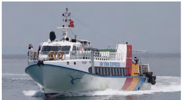
An Vinh Express... also propelled by dual 1,300 hp Cummins KTA38 engines.
