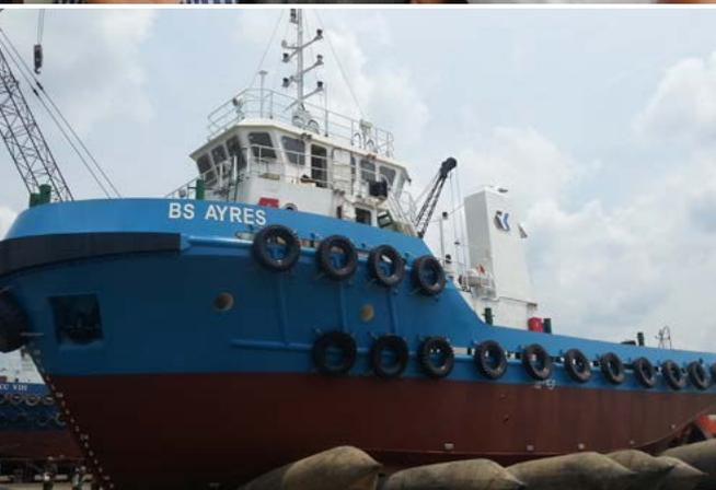
Top: 40-metre anchor handling tug (AHT) for oil and gas industry is powered by dual 2200 hp Cummins QSK60 MCRS engines.
